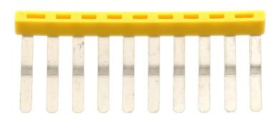
External insulated cross-connector, No. of poles: 10, Mounting type: Plug in, Width: 50.1 mm, Rated current: 27 A; Colour: Yellow
