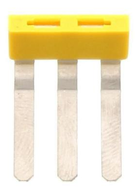
External insulated cross-connector, No. of poles: 3, Mounting type: Plug in, Width: 16.9 mm, Rated current: 27 A; Colour: Yellow
