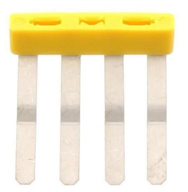
External insulated cross-connector, No. of poles: 4, Mounting type: Plug in, Width: 19.46 mm, Rated current: 27 A; Colour: Yellow
