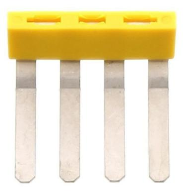
External insulated cross-connector, No. of poles: 4, Mounting type: Plug in, Width: 23 mm, Rated current: 27 A; Colour: Yellow
