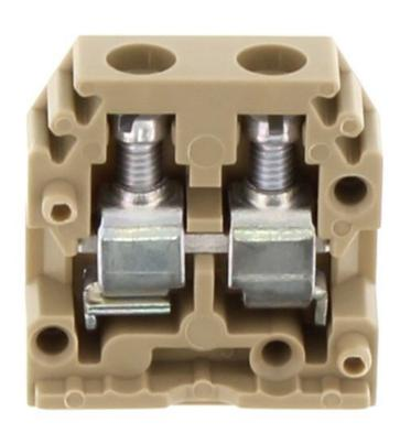
Feed-through terminal for direct mount, Screw connection, Mounting type: Mounting surface, Rated cross-section: 4 mm², Width: 6 mm, Colour: Beige
