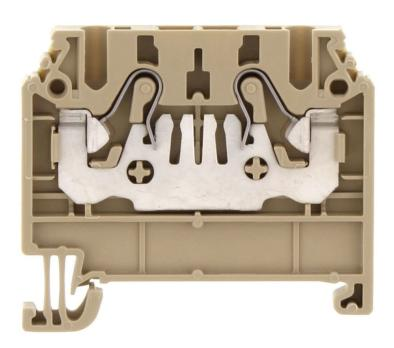
Feed-through terminal, Push-in connection, Mounting type: Mounting rail TS 35/7.5, Rated cross-section: 1.5 mm², Width: 4.1 mm, Colour: Beige
