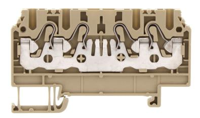
Feed-through terminal, Push-in connection, Mounting type: Mounting rail TS 35/7.5, Rated cross-section: 1.5 mm², Width: 4.1 mm, Colour: Beige
