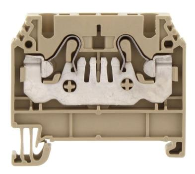
Feed-through terminal, Push-in connection, Mounting type: Mounting rail TS 35/7.5, Rated cross-section: 2.5 mm², Width: 5.1 mm, Colour: Beige
