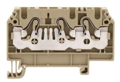
Feed-through terminal, Push-in connection, Mounting type: Mounting rail TS 35/7.5, Rated cross-section: 2.5 mm², Width: 5.1 mm, Colour: Beige
