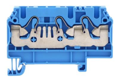
Feed-through terminal, Push-in connection, Mounting type: Mounting rail TS 35/7.5, Rated cross-section: 4 mm², Width: 6.1 mm, Colour: Blue
