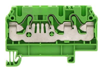
Feed-through terminal, Push-in connection, Mounting type: Mounting rail TS 35/7.5, Rated cross-section: 4 mm², Width: 6.1 mm, Colour: Green
