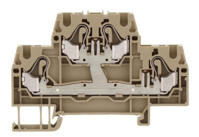
Double-level terminal, Push-in connection, Mounting type: Mounting rail TS 35/7.5, Rated cross-section: 2.5 mm², Width: 5.1 mm, Colour: Beige
