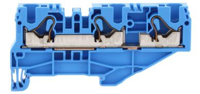
Feed-through installation terminal, Push-in connection, Mounting type: Mounting rail TS 35/7.5, Rated cross-section: 10 mm<sup>2</sup>, Width: 8.1 mm, Colour: Blue
