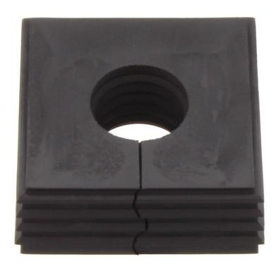
Seal, Mounting type: Plug in, Length x width: 42.8 mm, Max. cable diameter: 18 mm, IP 66, Colour: Black
