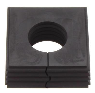
Seal, Mounting type: Plug in, Length x width: 42.8 mm, Max. cable diameter: 21 mm, IP 66, Colour: Black
