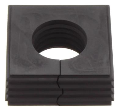
Seal, Mounting type: Plug in, Length x width: 42.8 mm, Max. cable diameter: 23 mm, IP 66, Colour: Black
