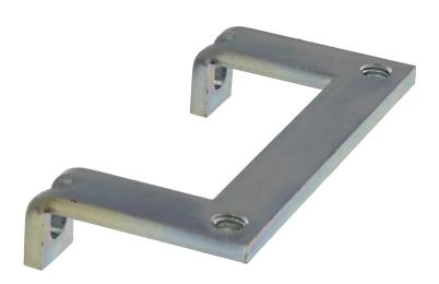
Shield-connection rail enabling mounting of shield connection clips directly on cable entry system KDS, Mounting type: Screw, Length: 35,3 mm, Width: 68 mm, Height: 16 mm, Profile: 10x3 mm
