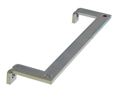
Shield-connection rail enabling mounting of shield connection clips directly on cable entry system KDS and KES, Mounting type: Screw, Length: 35,3 mm, Width: 140 mm, Height: 16 mm, Profile: 10x3 mm
