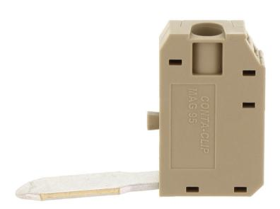
Measurement pick-off terminal, Screw connection, Mounting type: On base, Rated cross-section: 10 mm², Width: 10 mm, Colour: Beige
