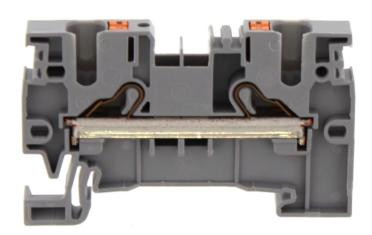
Feed-through terminal, Push-in connection, Mounting type: Mounting rail TS 35/7.5, Rated cross-section: 4 mm², Width: 6.1 mm, Colour: Grey
