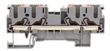
Feed-through terminal, Push-in connection, Mounting type: Mounting rail TS 35/7.5, Rated cross-section: 4 mm², Width: 6.1 mm, Colour: Grey
