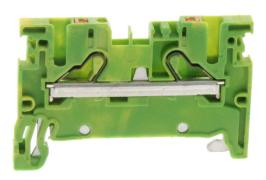
Protective earth terminal, Push-in connection, Mounting type: Mounting rail TS 35/7.5, Rated cross-section: 1.5 mm², Width: 3.5 mm, Colour: Green-yellow
