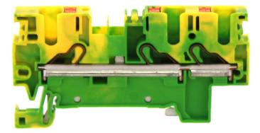
Protective earth terminal, Push-in connection, Mounting type: Mounting rail TS 35/7.5, Rated cross-section: 4 mm<sup>2</sup>, Width: 6.1 mm, Colour: Green-yellow
