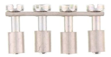
Cross-connector, No. of poles: 4, Mounting type: Can be screwed on, Width: 22.7 mm, Rated cross-section: 2.5 mm<sup>2</sup>, Colour: natural
