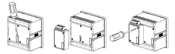
Connect the RI-F500/RI-F550 to the power supply, and then enter the module interface of the RI-F500/RI-F550 to check the information of slot X2. If the connection between the meter and the module is correct, the parameters of RI-A5RO5A will be shown.
