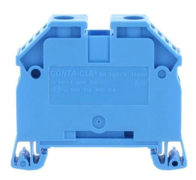
Feed-through terminal, Screw connection, Mounting type: Mounting rail TS 35/7.5, Rated cross-section: 16 mm², Width: 12 mm, Colour: Blue
