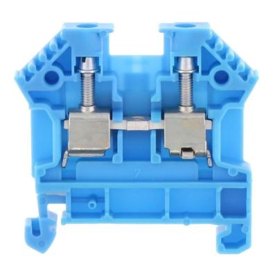
Feed-through terminal, Screw connection, Mounting type: Mounting rail TS 35/7.5, Rated cross-section: 4 mm², Width: 6 mm, Colour: Blue
