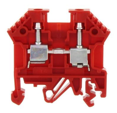
Feed-through terminal, Screw connection, Mounting type:Mounting rail TS 35/7.5 and TS 32, Rated cross-section: 4 mm², Width: 6 mm, Colour: Red
