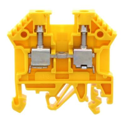
Feed-through terminal, Screw connection, Mounting type:Mounting rail TS 35/7.5 and TS 32, Rated cross-section: 4 mm², Width: 6 mm, Colour: Yellow
