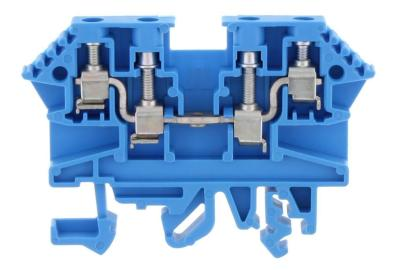
Feed-through terminal, Screw connection, Mounting type:Mounting rail TS 35/7.5 and TS 32, Rated cross-section: 4 mm<sup>2</sup>, Width: 6 mm, Colour: Blue
