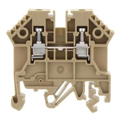
Feed-through terminal, Screw connection, Mounting type:Mounting rail TS 35/7.5, Rated cross-section: 2.5 mm², Width: 5 mm, Colour: Beige
