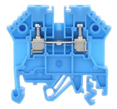
Feed-through terminal, Screw connection, Mounting type:Mounting rail TS 35/7.5, Rated cross-section: 2.5 mm<sup>2</sup>, Width: 5 mm, Colour: Blue
