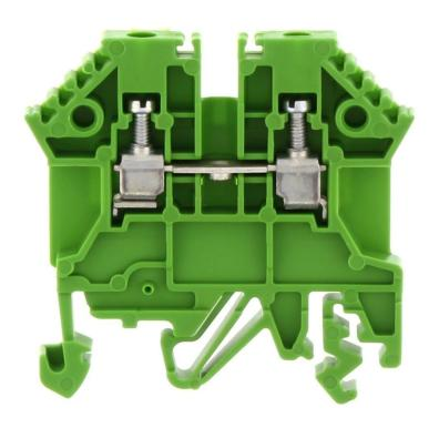
Feed-through terminal, Screw connection, Mounting type:Mounting rail TS 35/7.5 and TS 32, Rated cross-section: 2.5 mm², Width: 5 mm, Colour: Green
