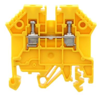
Feed-through terminal, Screw connection, Mounting type:Mounting rail TS 35/7.5 and TS 32, Rated cross-section: 2.5 mm<sup>2</sup>, Width: 5 mm, Colour: Yellow
