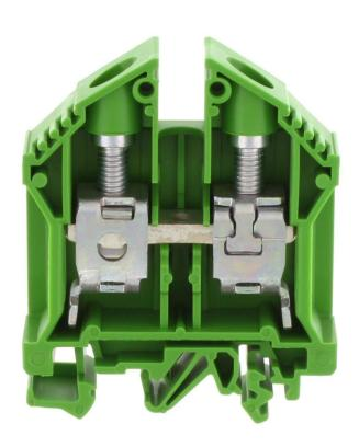
Feed-through terminal, Screw connection, Mounting type:Mounting rail TS 35/7.5 and TS 32, Rated cross-section: 35 mm², Width: 16 mm, Colour: Green
