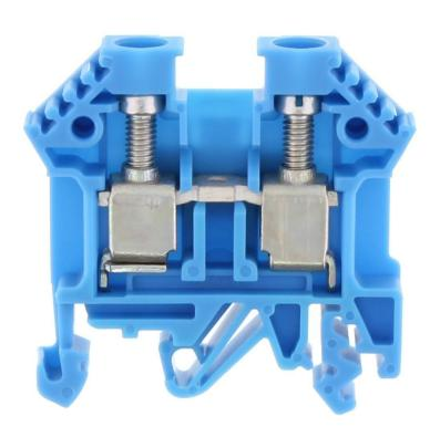
Feed-through terminal, Screw connection, Mounting type:Mounting rail TS 35/7.5 and TS 32, Rated cross-section: 10 mm², Width: 8 mm, Colour: Blue
