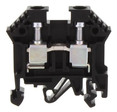
Feed-through terminal, Screw connection, Mounting type:Mounting rail TS 35/7.5 and TS 32, Rated crosssection: 10 mm<sup>2</sup>, Width: 8 mm, Colour: Black
