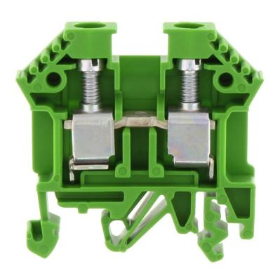
Feed-through terminal, Screw connection, Mounting type:Mounting rail TS 35/7.5 and TS 32, Rated cross-section: 10 mm², Width: 8 mm, Colour: Green
