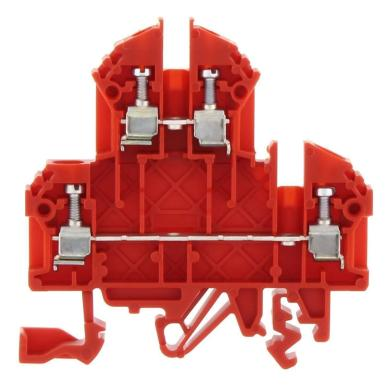
Double-level terminal, Screw connection, Mounting type:Mounting rail TS 35/7.5 and TS 32, Rated cross-section: 2.5 mm<sup>2</sup>, Width: 5 mm, Colour: Red
