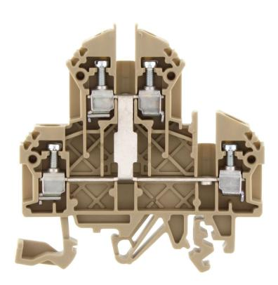
Double-level terminal, Screw connection, Mounting type:Mounting rail TS 35/7.5 and TS 32, Rated cross-section: 2.5 mm², Width: 5 mm, Colour: Beige
