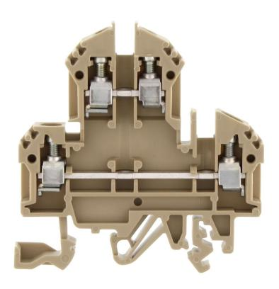
Double-level terminal, Screw connection, Mounting type:Mounting rail TS 35/7.5 and TS 32, Rated cross-section: 4 mm², Width: 6 mm, Colour: Beige
