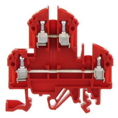
Double-level terminal, Screw connection, Mounting type:Mounting rail TS 35/7.5 and TS 32, Rated cross-section: 4 mm<sup>2</sup>, Width: 6 mm, Colour: Red
