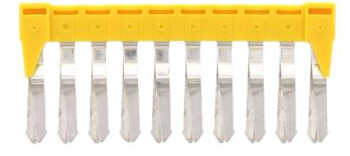
Insulated cross-connector, No. of poles: 10, Mounting type: Plug in, Width: 50.7 mm, Rated cross-section: 2.5 mm<sup>2</sup>, Colour: Yellow
