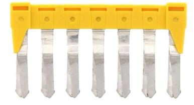
Insulated cross-connector, No. of poles: 7, Mounting type: Plug in, Width: 41.8 mm, Rated cross-section: 4 mm<sup>2</sup>, Colour: Yellow
