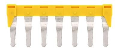
Insulated cross-connector, No. of poles: 7, Mounting type: Plug in, Width: 54.8 mm, Rated cross-section: 6 mm², Colour: Yellow
