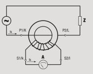
When connecting all amperometric transformers it is important to respect the directions of the current. Secondary: from S1/k to S2/l
