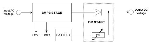
The **SMPS** stage is a switching mode power supply equipped with a plug battery in parallel that supplies a permanent output voltage of 13,8Vdc. Regarding this power supply, we use a quasi-resonant Flyback converter that improves emissions behavior and efficiency.
