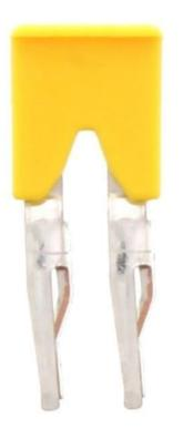
Insulated cross-connector, No. of poles: 2, Mounting type: Plug in, Width: 9.1 mm, Rated cross-section: 2.5 mm<sup>2</sup>, Colour: Yellow
