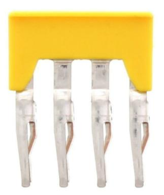
Insulated cross-connector, No. of poles: 4, Mounting type: Plug in, Width: 19.3 mm, Rated cross-section: 2.5 mm<sup>2</sup>, Colour: Yellow
