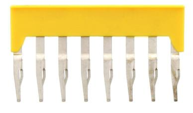
Insulated cross-connector, No. of poles: 8, Mounting type: Plug in, Width: 46.7 mm, Rated cross-section: 4 mm<sup>2</sup>, Colour: Yellow
